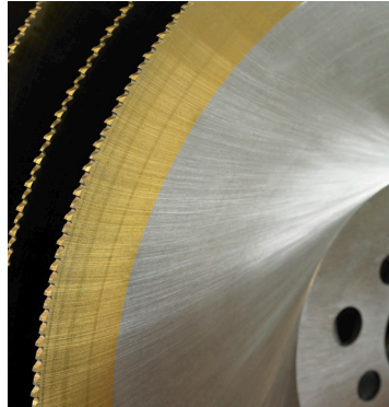
Resharpened: HSS metal circular saw blades
